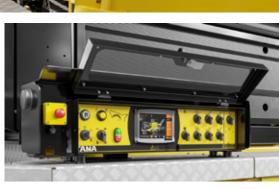
TCS with 12 pre-programmed operations, connected with TANA ProTrack\*.
