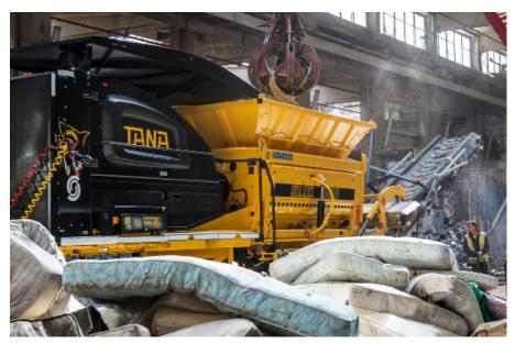
The slow-speed, single rotor TANA Shark shredder offers unique versatility. The robust TANA Shark is a great fit for difficult materials like tires and mattresses but also for various waste types like mixed, wood and construction waste.
