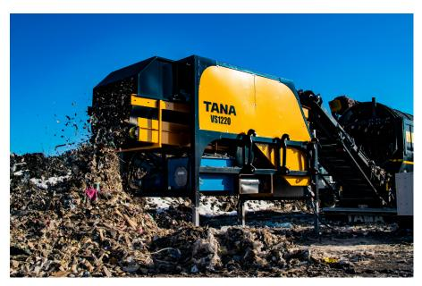
TANA VS1220 wind sifter separates light from heavy materials with a high grade of accuracy. It gives you more value by cleaning waste streams for further reuse or recycling.
