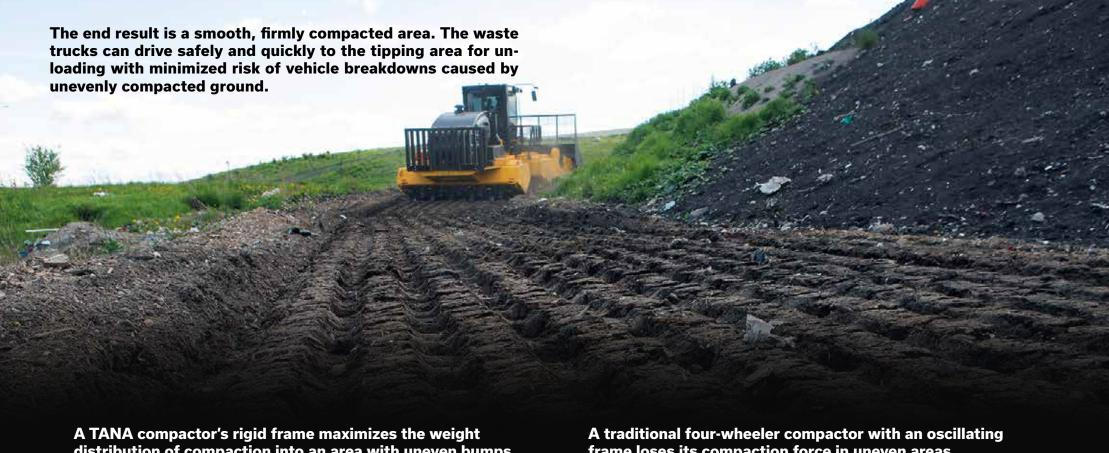
distribution of compaction into an area with uneven bumps.
