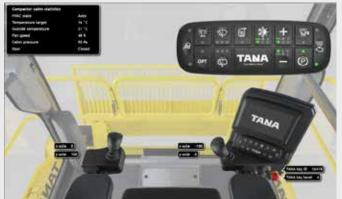
TANA ProTrack\* offers a tool for viewing the status of the compactor and details of the power pack components over the internet in real time.
