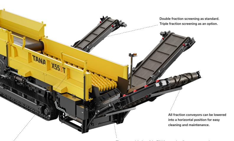
The side panels can be raised for cleaning and maintenance and to gain access to the modular screening deck for changing the particle size setting.
