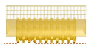
A traditional four-wheeler compactor with an oscillating frame loses its compaction force in uneven areas.
