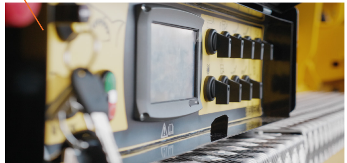
TCS with 12 pre-programmed operations, connected with TANA ProTrack®.
