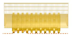
A traditional four-wheeler compactor with an oscillating frame loses its compaction force in uneven areas.
